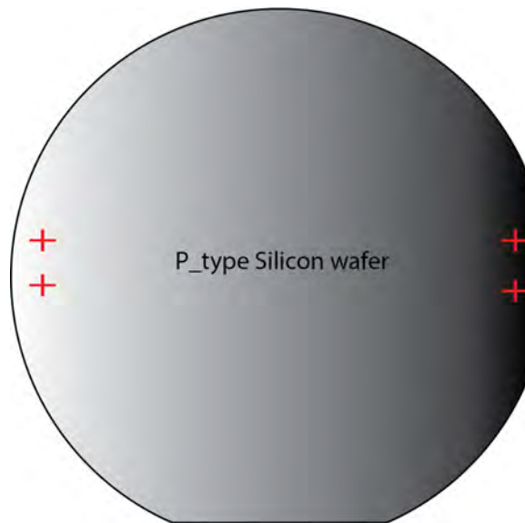
Figure 3.4: Zero alignment marks on the silicon wafer
