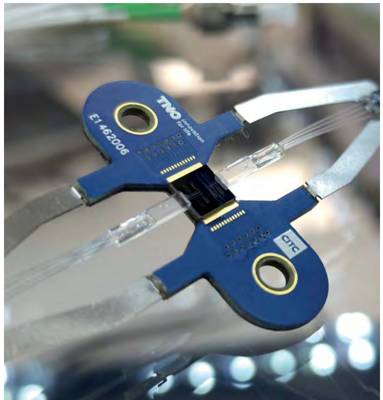
➤ Figure 1. Traditional way to optically couple to a PIC using direct attach fibre arrays units (FAUs). Such assemblies are suitable for companies seeking to assemble and package their (first) integrated photonic dies for prototyping. However, due to many discrete components involved, cumbersome footprints and loose fibres within the setup, such solutions are not suitable for mass-scale fabrication flows.
